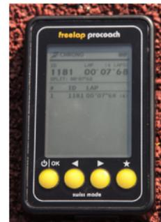
The Procoach is an handheld device that displays in LIVE lap time or time block per ID. The device can record up to 64 files and download onto a PC (Windows and Mac compatible).
