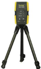
The Relay Coach collects the data from the FxChips as they pass a Tx Junior Pro transmitter set to FINISH mode. The data is then relayed to the Procoach handheld device, or an attached laptop, or a LED display.
