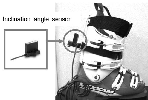
Fig. 3 Measurement of maximum lean angle using an inclination angle sensor
