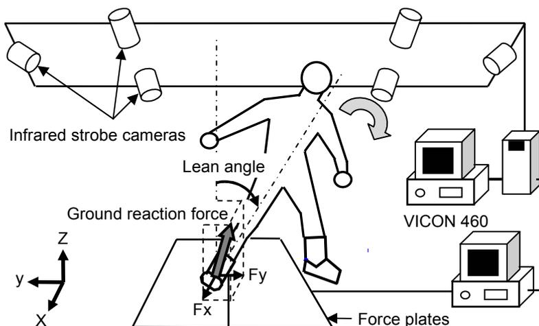
Fig. 5 Experimental apparatus for measuring of leaning balance
