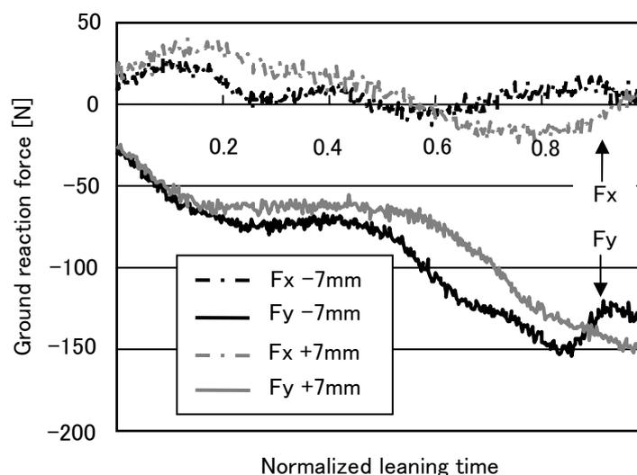
Fig. 7 Comparison of changes in ground reaction forces when leaning
