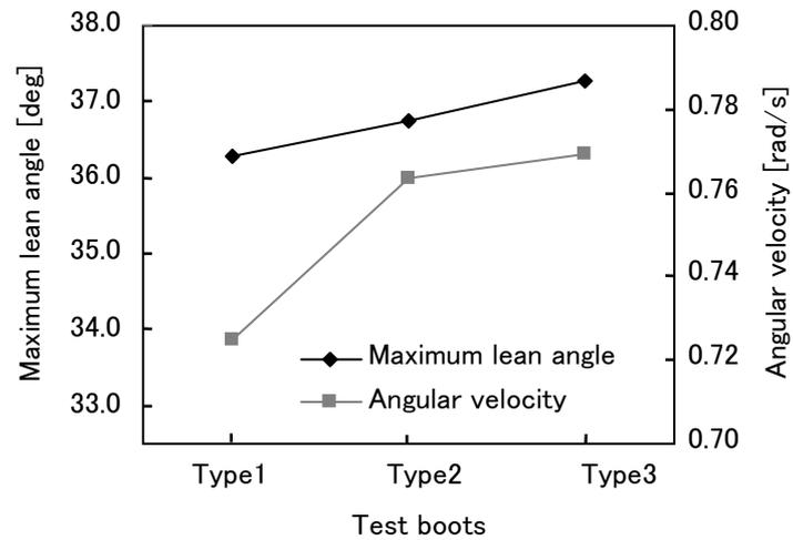
Fig. 9 Tests on effectiveness of upper shell design
