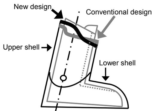
Fig. 8 New design of an upper shell based on leg frame
