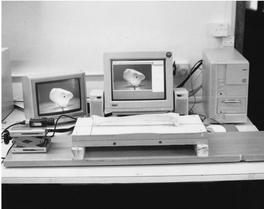
Fig. 4. Apparatus used to align the tibia and camera for the direct determination of the angle of tibial torsion.
